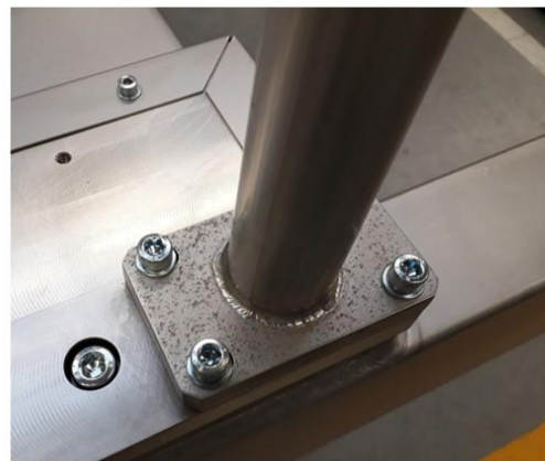
Bad blasted product
