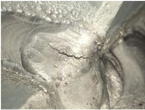
Crack in the weld
