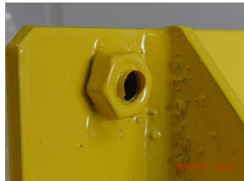
Threaded hole not lacquer free and welding spatters
