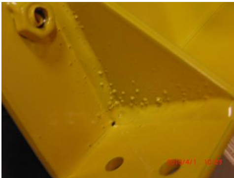
Holes and welding spatters
